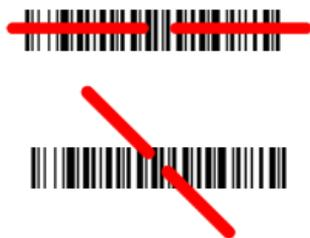
Hold the imager over the bar code, pull the trigger, and center the aiming beam on the bar code.
